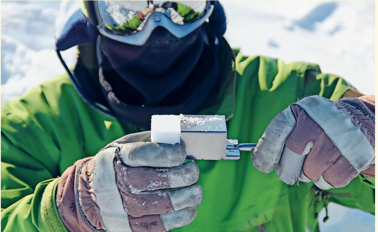
Even though the snow density data is recorded automatically, measurements by hand are still necessary – in often hostile conditions – to calibrate the instruments.
