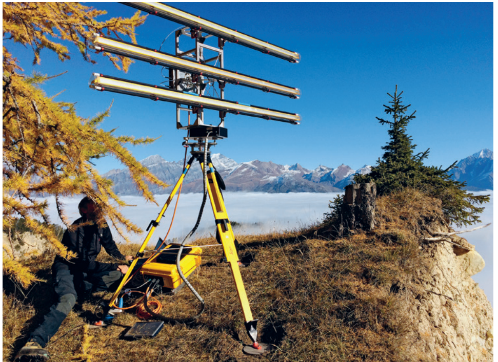
High above Illgraben, a radar measures the movements of landslides in the area. These landslides provide the material that makes up debris flows.
