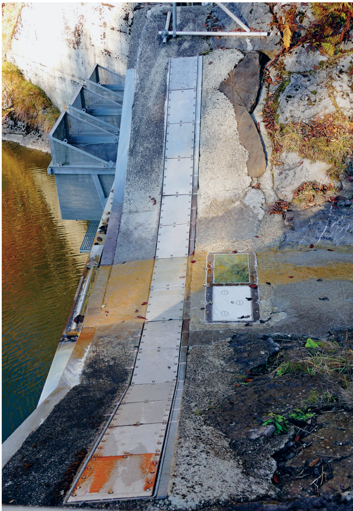
Geophones attached to the underside of these steel plates record vibrations and measure transport of coarse sediment on a continuous basis. The three metal collecting baskets are drawn automatically one after the other into the heavy flow of water.
