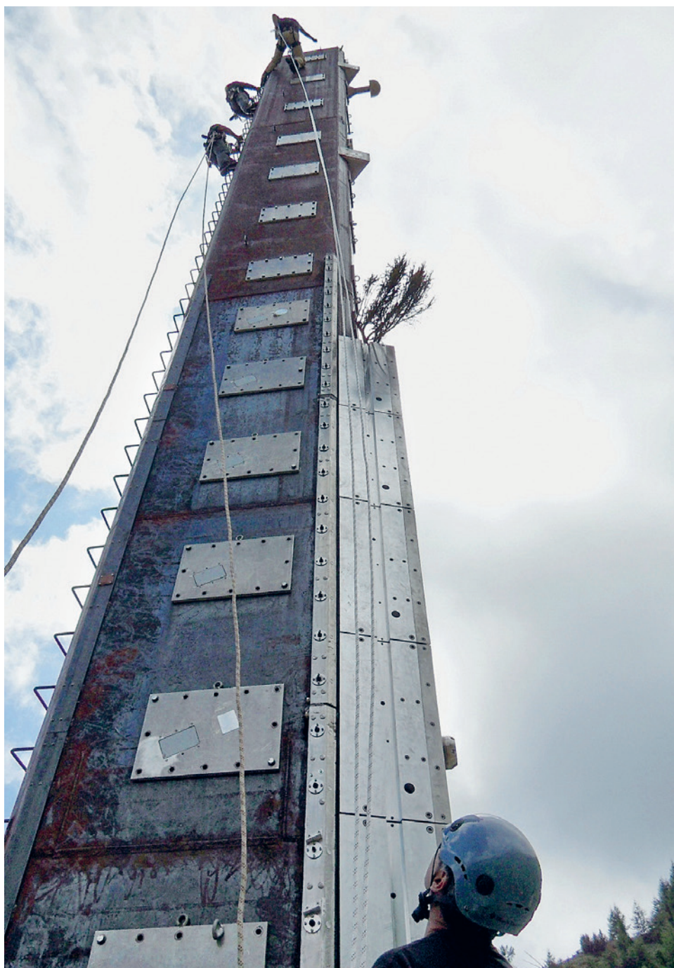
A 19-meter measurement tower in the middle of an avalanche track in the Vallée de la Sionne. It has a number of measurement devices to check the speed, pressure, density and temperature of an avalanche.
