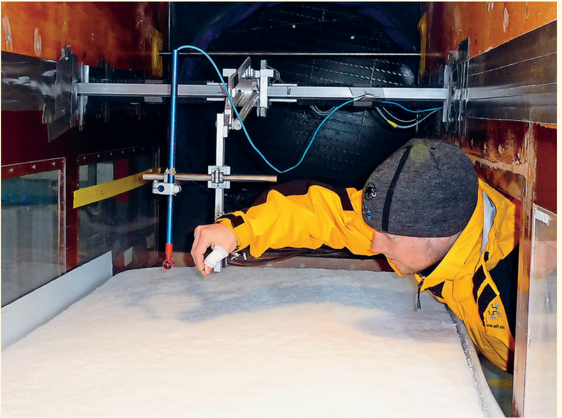
In the SLF's wind tunnel, researchers can study the transport of snow.
