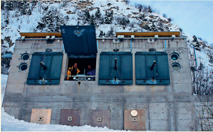
Researchers in the observation bunker use GEODAR, a radar system, to analyze the flow behavior of avalanches.
